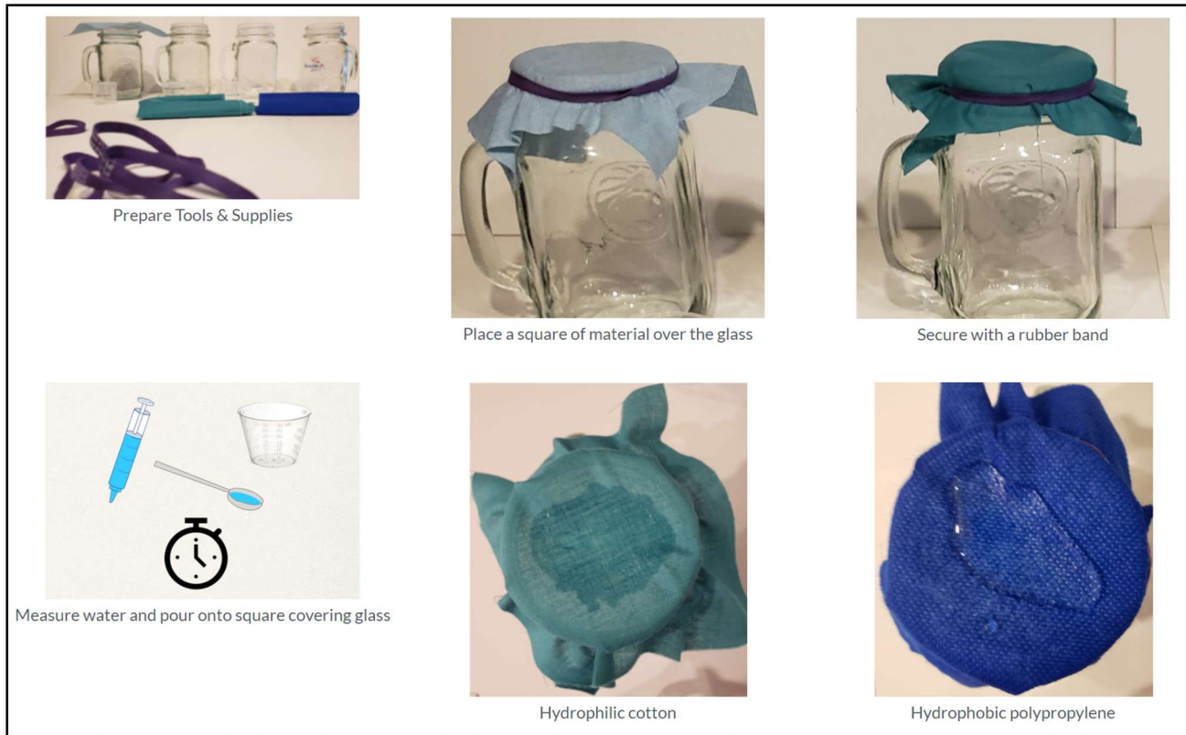
Figure 6 - Overview of MakerMask.org Water Resistance Test [12]
